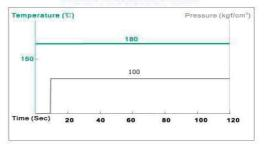
传压参数根据不同设备及产品规格需作相应调整;采用快压方式,后固化条件是 155-165℃、60-90 分钟。 The parameters of hot Pressure need to be adjusted according to different equipment and product specifications. After fast press, the curing condition is 150-160℃ for 60-90min.
